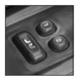
Your vehicle may have this feature. The controls are located on the driver's door, and are used to program and recall memory settings for the driver's seating positions, outside mirror positions and adjustable pedals (if equipped).
